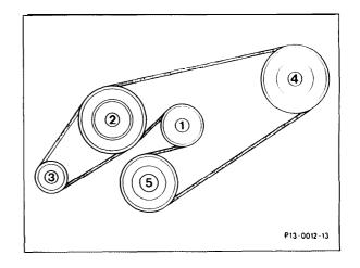
C Pulley layout on vehicles with power steering and refrigeration compressor
