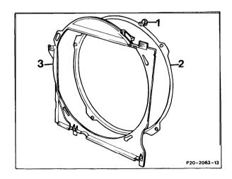
3 On engines 602 and 603 in model 124 Detach fan shroud and lay on the fan. Unscrew Viscofan coupling with fan and remove with fan shroud.
