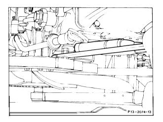
5 Detach tensioner, by unscrewing nut (378). Put a lever (12-13 mm dia., approx. 300 mm long) or rim wrench from vehicle tool kit in the hole in the spring tension lever (374). Press lever slightly to the left, until bolt (375) can be slid back in the direction of the manifold.
