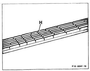
M Transverse cracks on the back.
