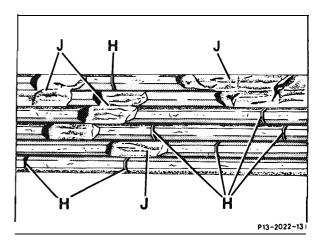
H Transverse cracks in several ribs.
