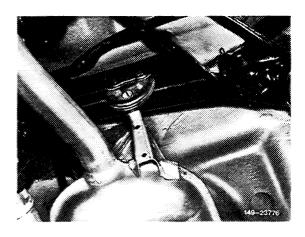
7 Mount sinter-sealing ring (5) on flange connection and pay attention to correct seat. Tightening torque of self-locking hex. nuts 20 Nm.
