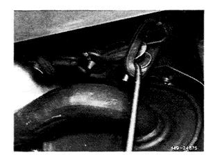
9 Mount rear damper in such a manner that the holding clamp of the rear damper is approx. 10 mm in front of holders on frame floor, so that the correct installation position is assured (arrows) in the event of an elongation of exhaust system.
