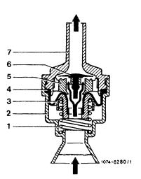
Vent valve opened at underpressure (vacuum)
