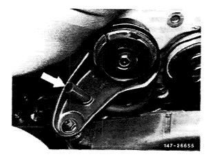
7 Unscrew fastening nuts for fuel tank and pull out drain hose (arrows) in upward direction in such a manner that hose can be installed behind edge of fuel tank. Slightly lift fuel tank for this purpose.
