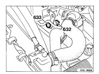
6 Screw down nut (632), withdraw bolt (633).
