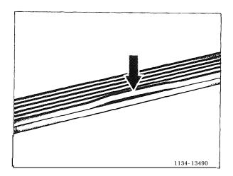
Cracks across the ribs (H) and/or sections of ribs broken off (J).
