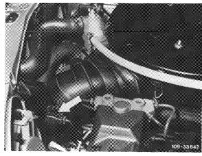
The intake scoop is attached with a spreader clip (1) and locked twice.
