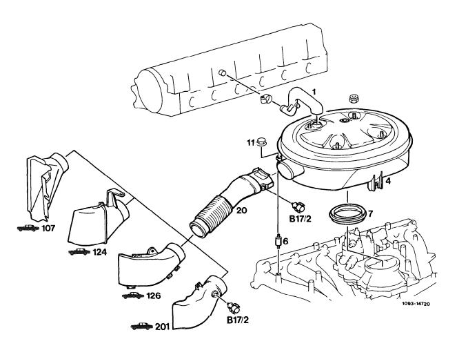
Intake air temperature sensor (B17/2)......
