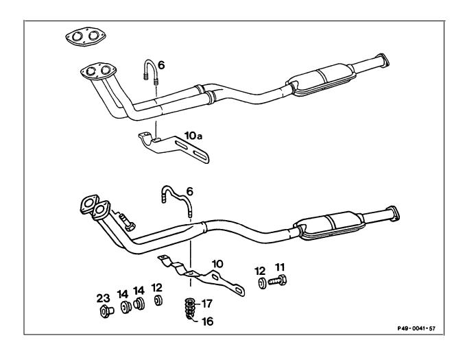
Pipe shackle (6) with **Belleville** spring washers (17) and self-locking nuts (23) ......
