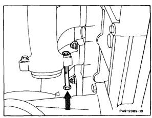
Insert new rivet nut into hole of exhaust manifold. Screw in caulking bolt and tighten to a torque of 30 Nm.
