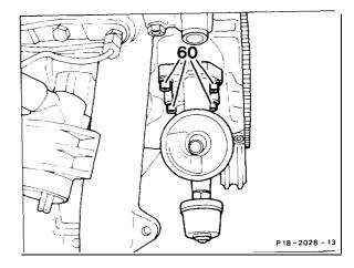
5 Clean sealing surfaces on oil filter and crankcase.
