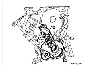
4 Remove oil pump gears, insert, oil with engine oil for this purpose.
