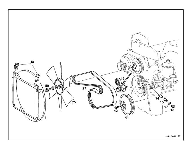
Screw plug (16) ...... unscrew, screw on, special tool
