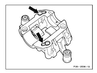
The rocker arm bearing points are lubricated from the longitudinal passage (a) in the cylinder head and the hydraulic valve clearance compensating elements supplied with oil (b) from there through a passage in the rocker arm.
