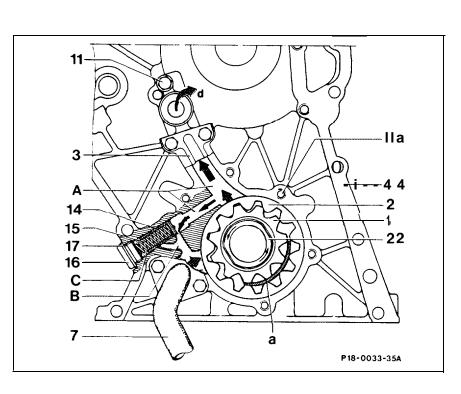
The teeth mesh again at the end of the pressure chamber and force the oil out of the tooth gaps.
