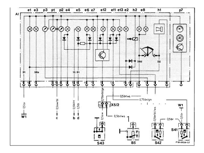
Wiring diagram engine oil level indicator, engine coolant level indicator, windshield washer level indicator
