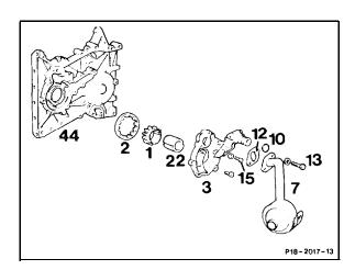
The sealing ring (12) seals the connection fitting at the oil pump cover (oil feed) to the oil passage in the crankcase.
