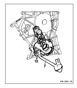
3 Unbolt oil pump cover, bolt on, replace Oring (10).
