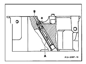
Part of the oil flows through the restriction passage (g) with dia. of 2.5 mm and the two grooves (arrows) in the rear rocker arm bearing bracket to the rear camshaft bearing and there into the hollow-drilled camshaft. The oil flows through the camshaft to the other camshaft bearings (flow-oriented oil feed).
