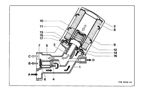
The two check valves (9-12 and 13-16) prevent the filter cartridge from running empty when the engine is switched off and when changing the filter.
