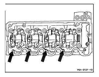
In the crankcase, the oil flowing back is passed along an oil collecting gallery (arrows) to the cast return passage.
