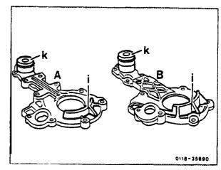
The drive sleeve for oil pump is manufactured from sintered metal, previously from steel.
