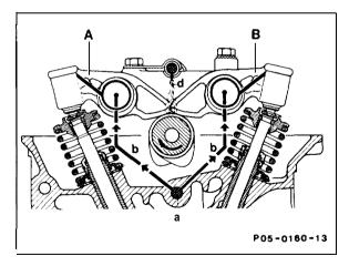
Lubrication of idler gear shaft and ignition distributor drive
