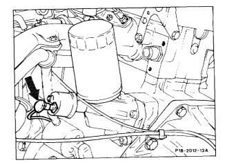
4 Unscrew oil filter base section, screw on, tightening torque 25 Nm.
