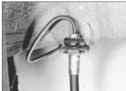
11.2 Rigid pipe-to-flexible hose connection
