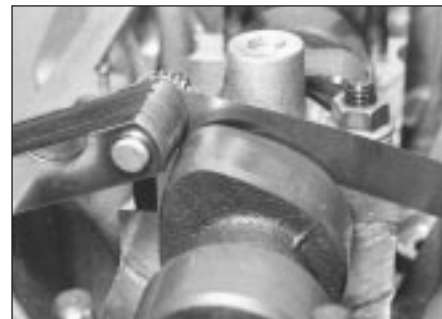
8.6 Measuring camshaft endfloat
