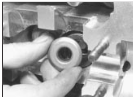
5.10 Removing valve spring upper seat
