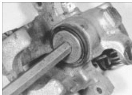
2.20a Retracting caliper piston using an Allen key
