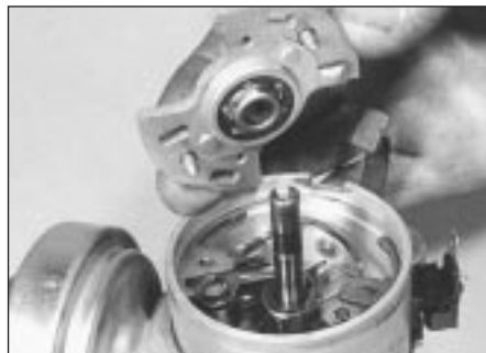
16.3 Removing the bearing plate - 1.05 and 1.3 litre
