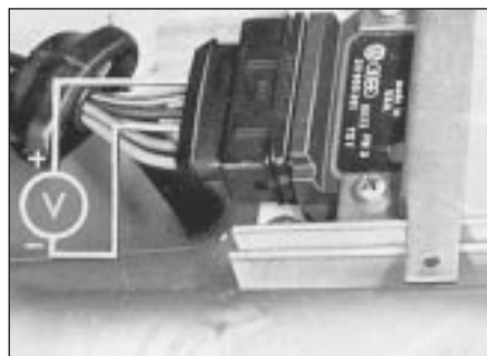
5.4 Voltmeter connection when testing Hall sender
