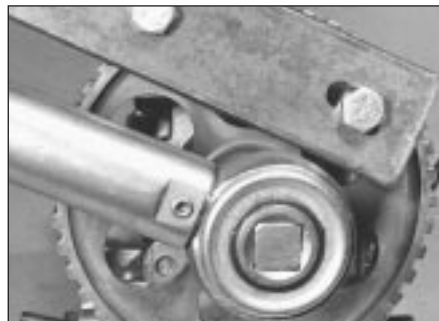
35.5 Method of tightening camshaft sprocket bolt
