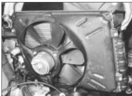
3.8 Lifting out radiator and cooling fan assembly
