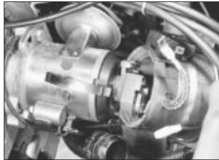
11.2 Withdraw distributor cap and screen ring
