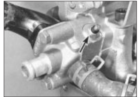
7.12 Temperature sensor (arrowed) - 1.05 and 1.3 litre
