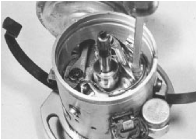
16.10b Adjusting contact breaker points gap
