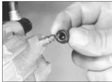
12.23 Fit bleed valve the protector cap
