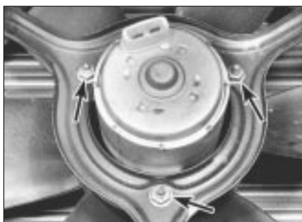
4.4 Cooling fan motor retaining nuts (arrowed)
