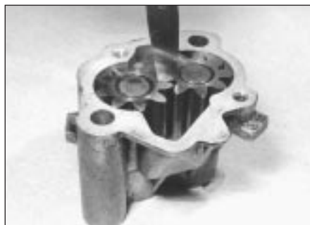
25.3 Checking oil pump gear backlash
