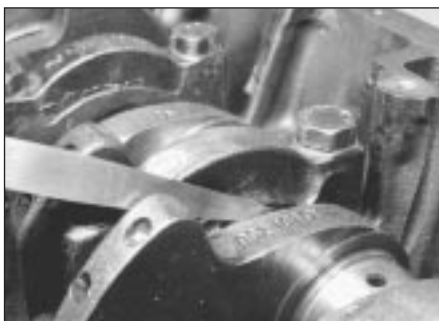
18.3 Checking crankshaft endfloat
