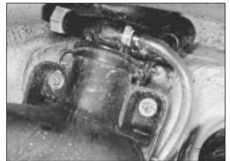
7.6 Fuel filler breather valve and hose
