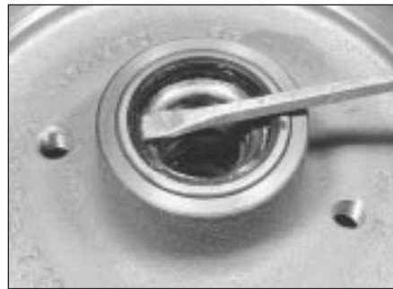
8.3 Prising out brake drum oil seal
