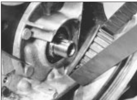
36.9 Fitting crankshaft sprocket and timing belt
