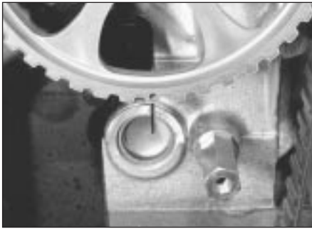
35.9 Camshaft sprocket (later type) with index mark aligned with timing cover TDC pointer
