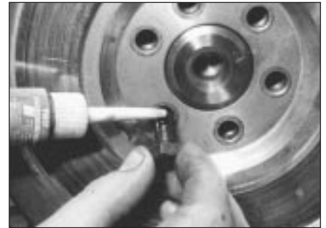
33.3 Applying liquid locking fluid to flywheel bolts
