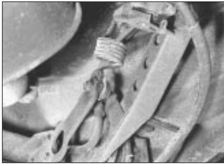
9.3 Brake pressure regulator unit showing spring bracket
