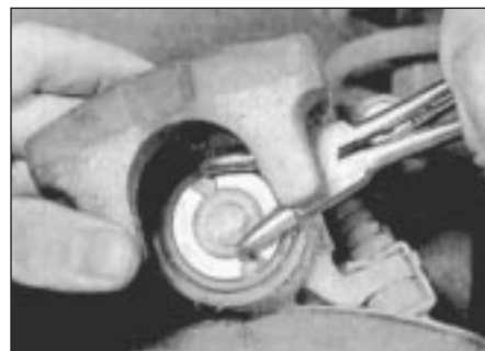
2.20b Retracting caliper piston using a pair of angled circlip pliers
