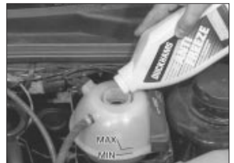
2.13 Topping-up engine coolant
