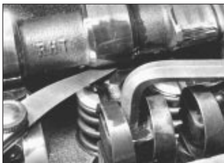
12.4 Adjusting a valve clearance - 1.05 and 1.3 litre
