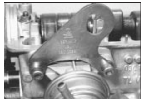
11.7b Location of engine lifting eye
