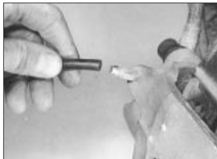
12.5 Connect bleed tube to bleed valve
