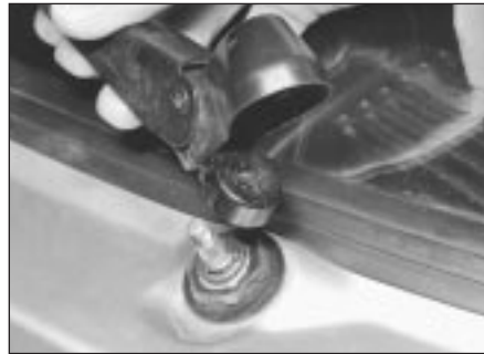
26.3 . . . and withdraw arm from spindle
