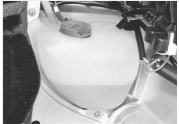
30.2 Rear window washer reservoir unit location
