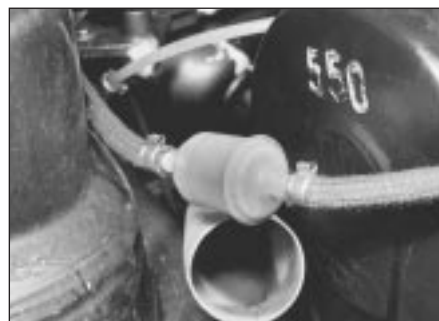
33.1 In-line fuel filter - 1.05 and 1.3 litre, carburettor
