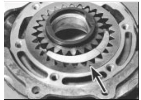
24.3b Outer rotor indentation (arrowed) must face cover
