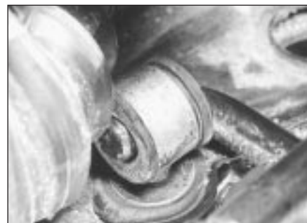
4.5 Anti-roll bar location in eye bolt
