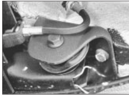
9.7 Axle beam pivot bolt head fitting position
