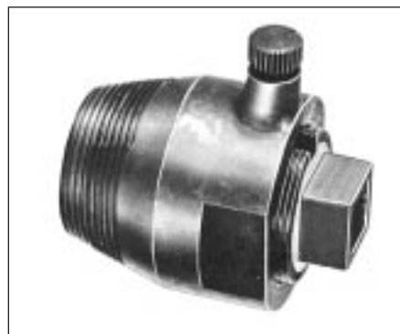
20.8 VW tool 2085 for removing crankshaft oil seal (timing belt end) and camshaft oil seal
