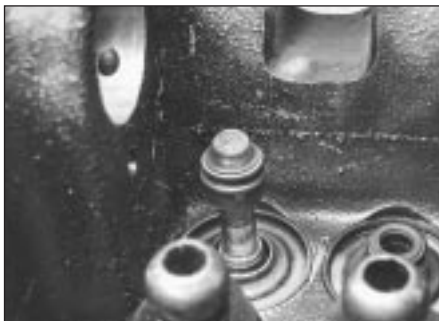
34.4 . . . then fit the new oil seal
