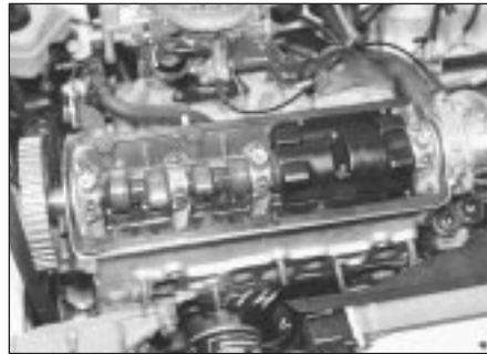
11.17 Plastic oil shield correctly located
