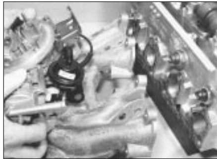
11.2b Fitting inlet manifold complete with carburettor
