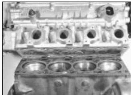
9.9 Removing cylinder head . . .
