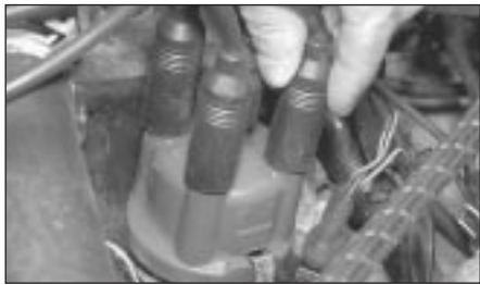
A Check that the HT lead connections at the distributor are clean and make sure they are secure by pushing them onto the cap.
