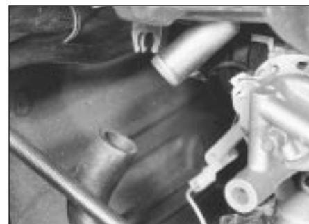
3.3b ... and crankcase emission hose - 1.3 litre
