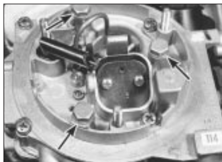
13.8 Carburettor securing bolts (arrowed) - Pierburg/Solex 2E3
