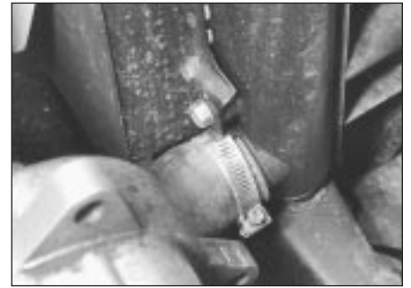
2.4b Radiator bottom hose connection - 1.8 litre
