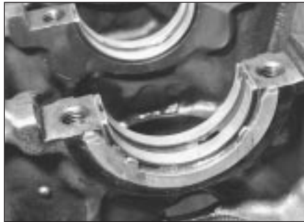
29.3 Thrustwasher location on centre main bearing
