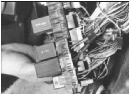
3.5 Fuse/relay unit removal, showing rear connections
