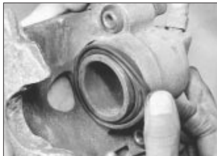
3.5 Removing the dust seal
