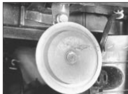
24.1a Single horn location behind front grille
