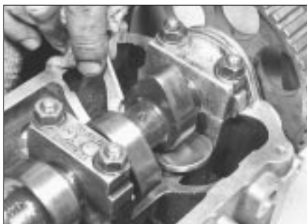
12.12 Removing a tappet bucket shim - 1.6 and 1.8 litre
