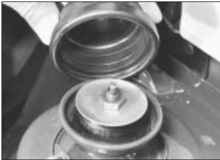
8.4 Removing rear suspension strut top cap
