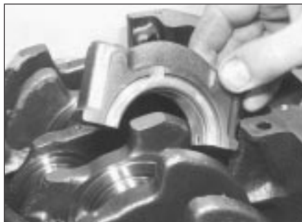
30.5 Fitting main bearing caps
