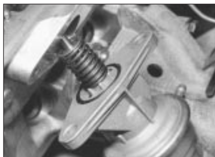
11.7a Fitting fuel pump
