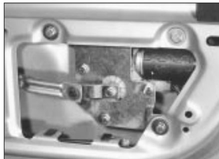
28.4b Rear wiper motor mounting in tailgate
