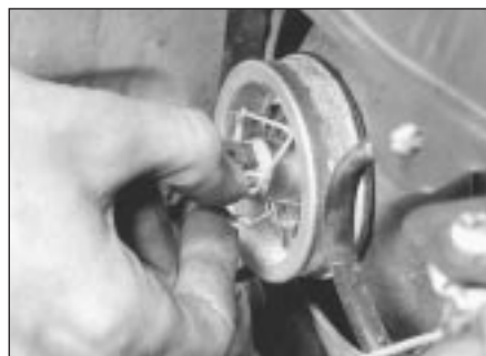
4.3 Squeeze bulb retaining clips . . .
