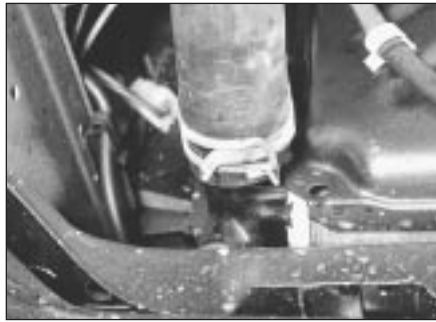
2.4a Radiator bottom hose connection - 1.3 litre
