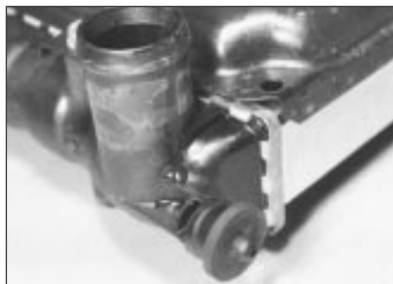
3.13 Radiator lower mounting rubber
