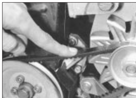
13.2 Checking alternator drivebelt tension
