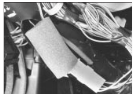
12.7b Additional under dash wiring connection and insulator - GTi
