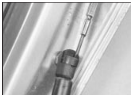
9.2a Releasing tailgate strut balljoint clip
