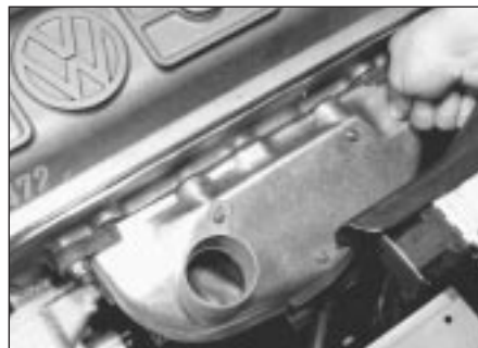
11.20 Fitting hot air shroud
