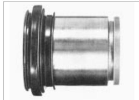
3.9 Dust seal location on caliper piston
